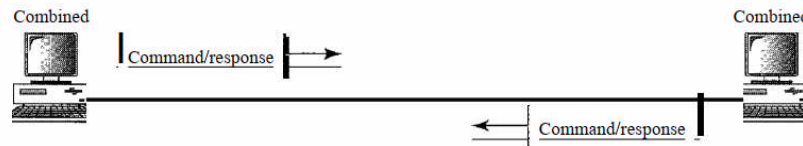
Figure 8.14: Asynchronous Balanced Mode
