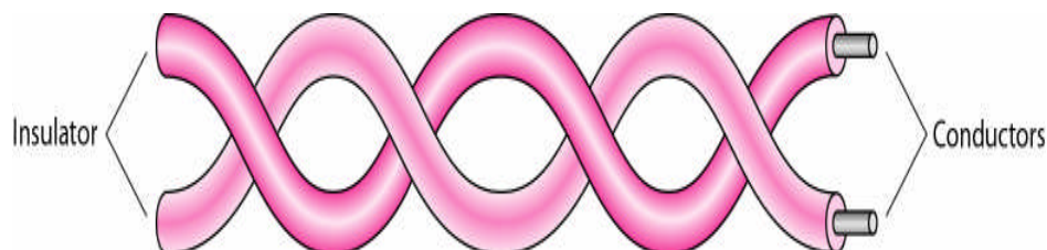
Figure 6.3: Twisted – pair cable
