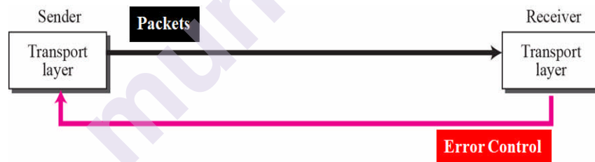
Figure 15.8: Error control at Transport layer
