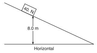
If 50. joules of heat is generated as the block slides down the incline, the maximum kinetic energy of the block at the bottom of the incline is
