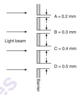
Which opening will cause the greatest diffraction?
