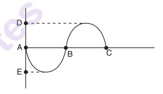
The distance between which two points identifies the amplitude of the wave?
