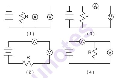
44 Identical resistors (R) are connected across the same 12-volt battery. Which circuit uses the greatest power?
