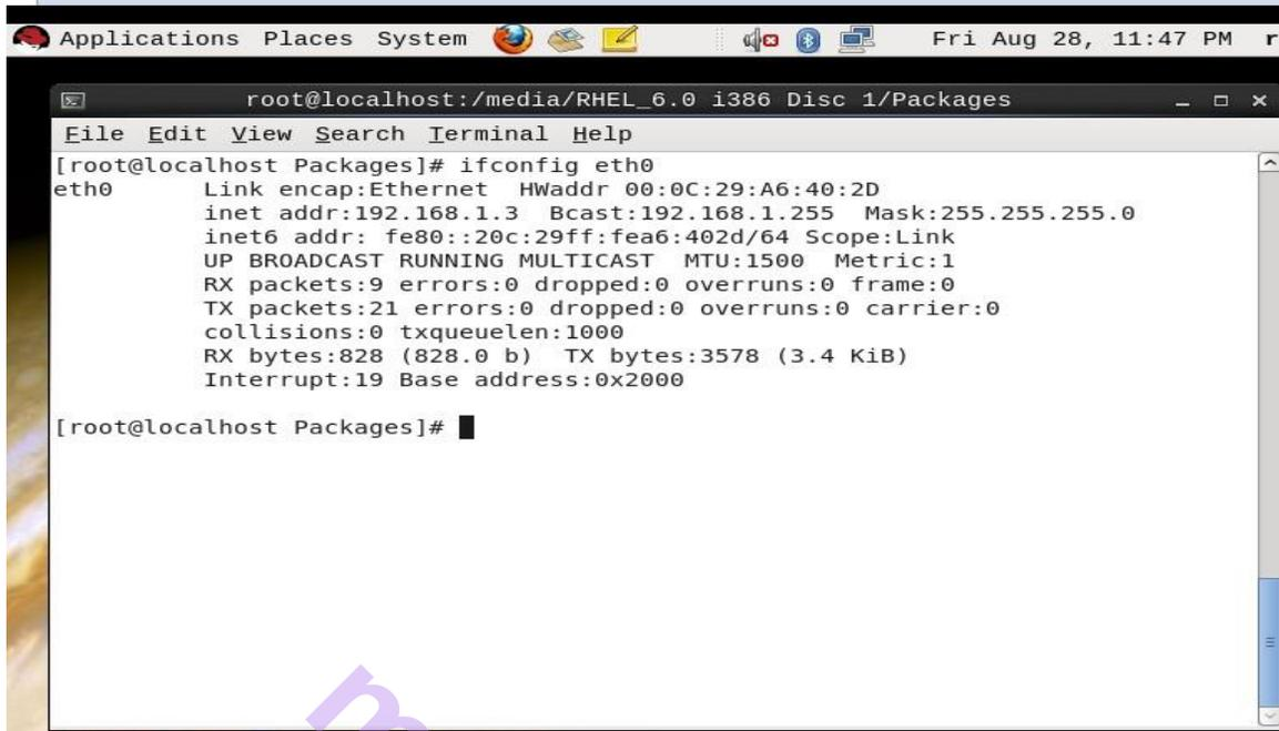
A terminal window titled 'root@localhost:/media/RHEL\_6.0 i386 Disc 1/Packages' showing the output of the 'ifconfig eth0' command. The output displays network configuration details for the eth0 interface, including IP address, netmask, broadcast address, and various statistics.
