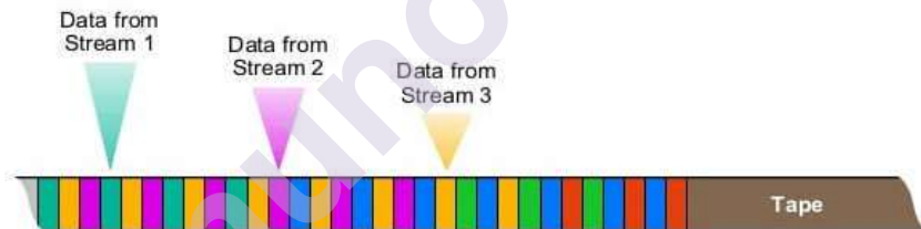
Figure 9-16 Multiple streams on tape media
