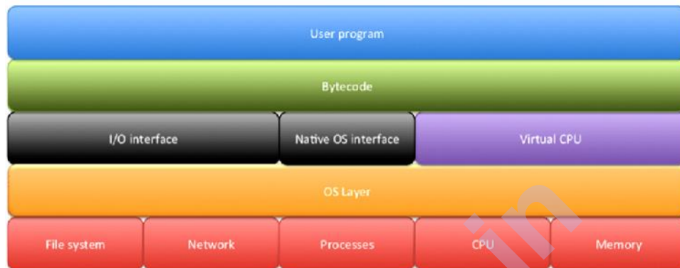
Figure 1.15 process virtual machine design Reference from “Mastering Cloud Computing Foundations and Applications Programming” by Rajkumar Buyya)
