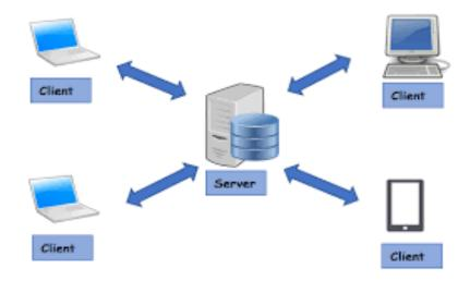
The **clients to server network communicate** with each other through a centralized server If Client 1 wants to send data to Client 2, it first sends a request to the server for permission. The server sends a signal to client 1, from which communication can be initiated.
