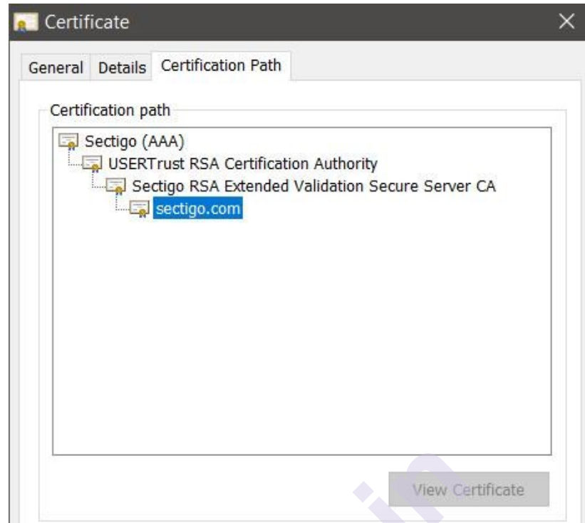
Figure: SSL/TLS certificates often combine intermediate certificates to create a hierarchical trust chain
