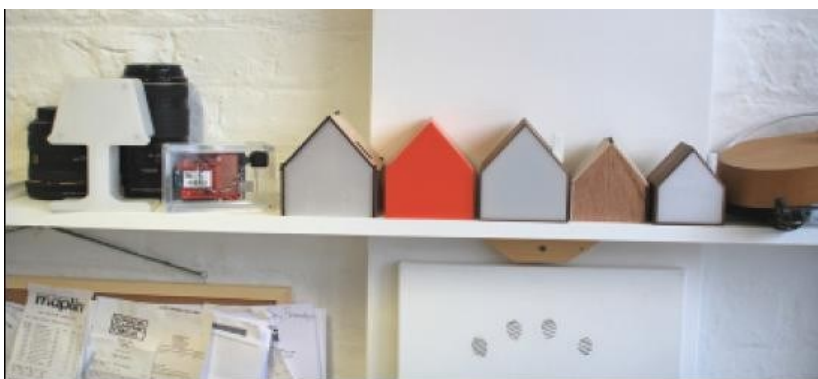
The evolving design for the Good Night Lamp (from left to right): original design; functional mockup; redesign mockup; redesign functional prototypes (orange and wood/acrylic); revised size mockup; revised size functional prototype.
