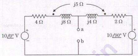
Obtain Norton equivalent circuit at terminals ab of the coupled circuit shown in the figure. Using it, find out the current passing through 5  $\Omega$  resistor connected between the terminals ab.
