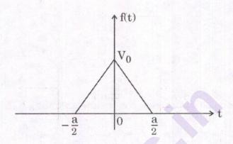
The figure shows a triangular pulse which is zero for all time except  $-\frac{a}{2} \le t \le \frac{a}{2}$ . For this pulse
