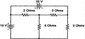
b) Find I<sub>2</sub>(S) for the following transformed circuit and hence find i<sub>2</sub> (t) using Inverse Laplace Transform.
