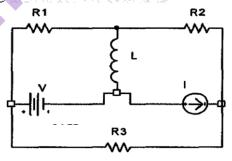
2. a) For the circuit shown below, find the current through 3 ohms resistor, using superposition theorem.
