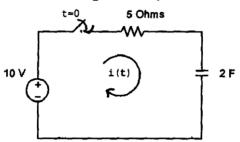
c) Find the driving point impedance for the following network.
