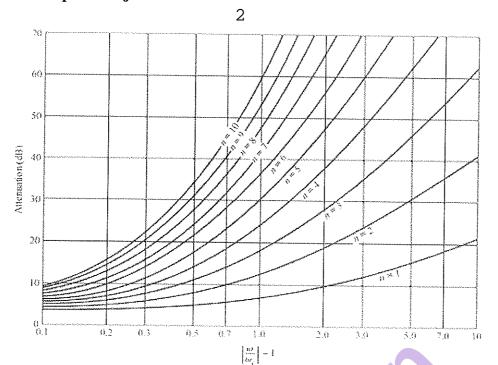
Attenuation versus normalized frequency for maximally flat filter prototypes. Adapted from G. L. Matthaet, L. Young, and E. M. T. Jones, Microwave Filters, Impedance-Matching Networks, and Coupling Structures, Artech House, Dedham, Mass., 1980, with permission.
