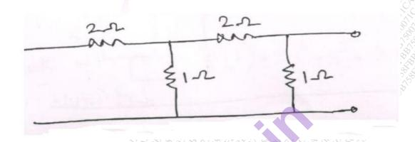
d) Find nominal impedance, cut-off frequency and passband for the network shown.
