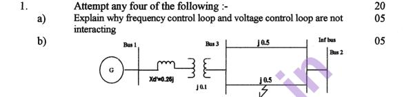
For the system shown if fault occurs at the middle of the line. Find transfer reactance between bus 1 and 2 by **NODE ELIMINATION** technique only
