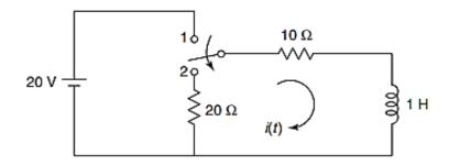
5. (A) In the given network of figure, the switch is opened at t = 0. Solve for V, dv/dt and  $d^2v/dt^2$  at  $t = 0^+$ .
