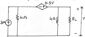
3(a) In the network shown in figure at t=0, the switch is opened. calculate v, dv/dt and  $d^2v/dt^2$  at  $t=0^+$
