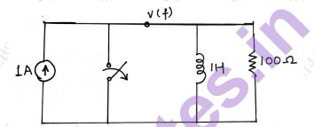
(b) In the network shown in figure the switch is closed and steady state is attained. At at t=0, switch is opened. Determine the current through the inductor.
