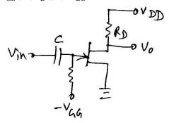
(c) In JEET circuit show with self bias  $V_{DD} = 25V$ ,  $R_D = 3kW$ ,  $R_S = 400W$ , ID = 2.mA (05) Determine  $V_{DS}$  and  $V_{GS}$
